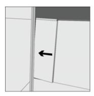
Push the panel into the edge trim channel while laying the panel down toward the substrate.
