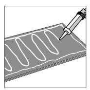
Apply the panel to the substrate by pressing it into place. Apply even pressure with your hands across the entire panel. If necessary, use shims or pins to hold panels in place until the adhesive sets.
