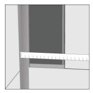
After cutting the panel to length, apply adhesive in a zig zag pattern to the back of the panel or on substrate.
