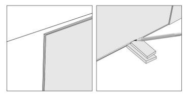
Apply adhesive to the back of the panel. Carefully read and follow the adhesive manufacturer's directions. Apply a 1/4-inch / 6mm bead of adhesive in a zigzag pattern, and a bead around the panel perimeter about 1 inch / 25mm from the edges, or apply by troweling the adhesive onto the substrate, following your adhesive manufacturer's recommendations.
