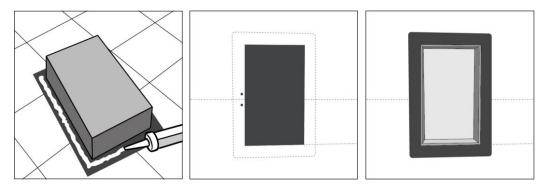
For niches that fit over your new Wall Tile installation, finish your installation around the niche opening, installing so that the tile edges are flush with the niche opening edges of the substrate. Insert your preformed niche and apply sealant to all edges where the niche meets the surface of your Wall Tiles.
